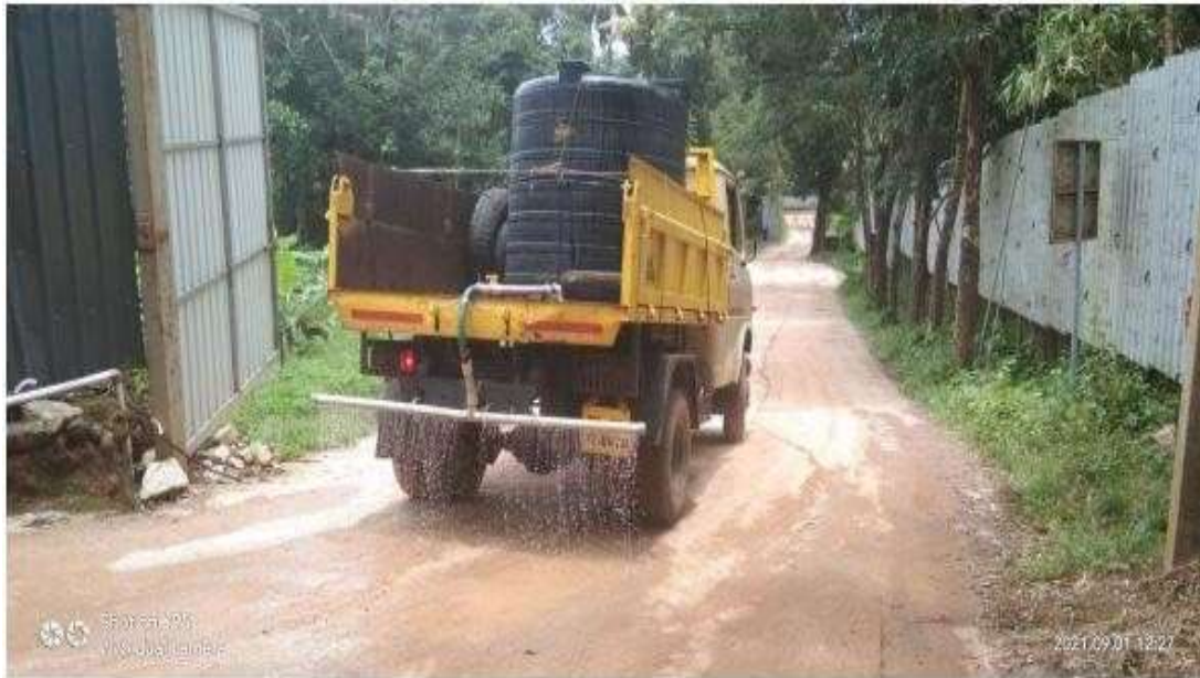
Figure 3: Photographs showing water spraying on quarry road for dust suppression.
