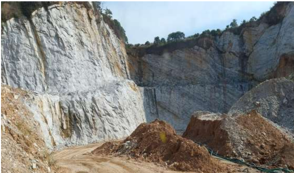
Figure 7: Photographs showing bench development / Mining face development
